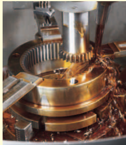
Gear cutting by CNC Gear Shaper
